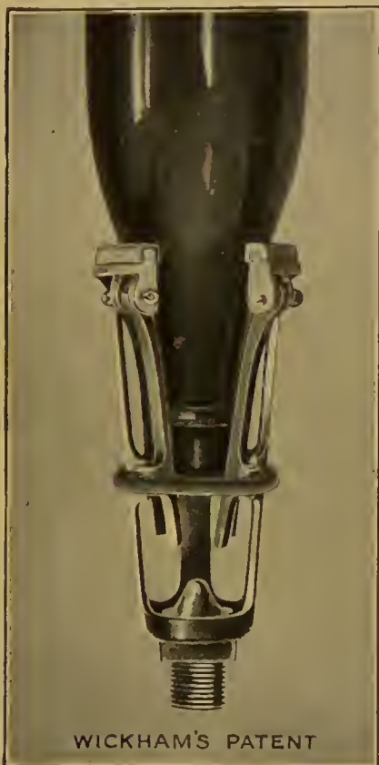
FIG. 95.—Wickham's Patent Rinsing Mechanism with Bottle in Position.
